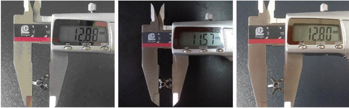
Figure 2. Measurement of EVA samples by electronic vernier calipers.
