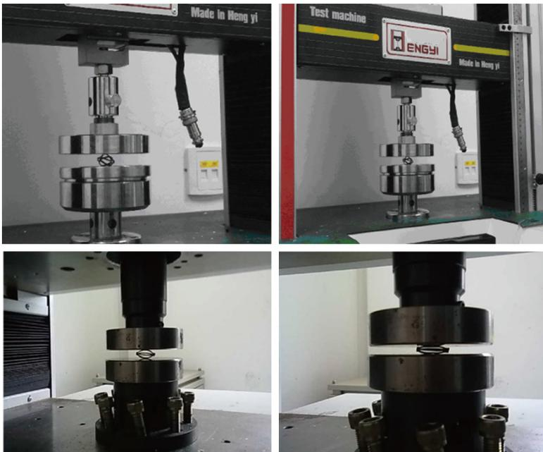
Figure 3. The biomechanical testing of EVA.
