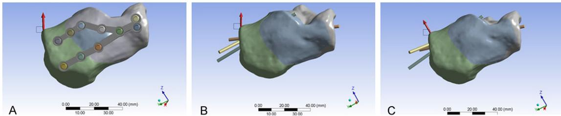
**Figure 2.** A vertical force of 160 N was applied on the fractured calcaneus via the Achilles tendon at 0° (neutral position) for plate group (A), and at 0° (neutral position) and 30° (plantar flexed position) for multi-pin group (B&C), respectively.
