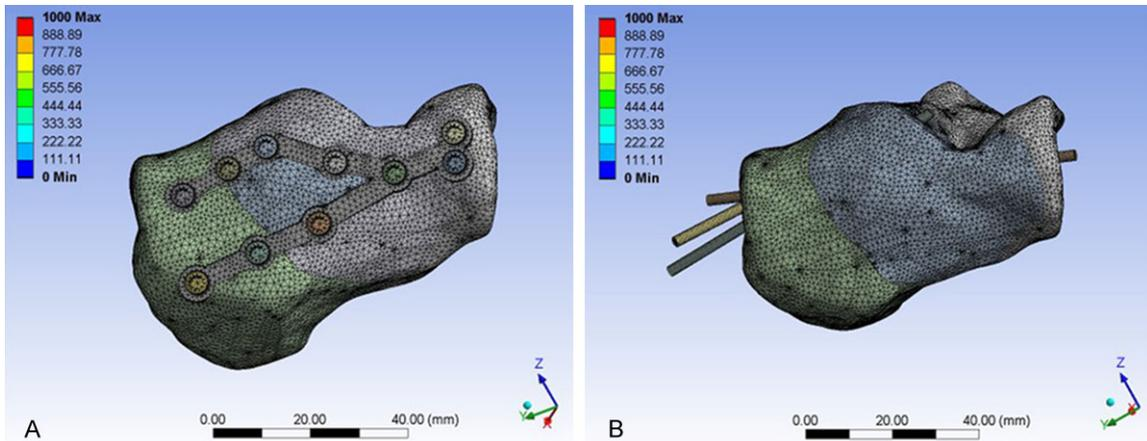
**Figure 1.** Three-dimensional finite element model of plate fixation (A) and multi-pin fixation for calcaneal fracture (B).
