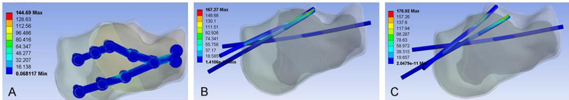
**Figure 4.** The von Mises stress at 0° (neutral position) for plate group (A), and at 0° (neutral position) (B) and 30° (plantar flexed position) (C) for multi-pin group.
