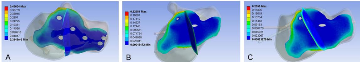
**Figure 5.** The equivalent strain of fracture line at 0° (neutral position) for plate group (A), and at 0° (neutral position) (B) and 30° (plantar flexed position) (C) for multi-pin group.
