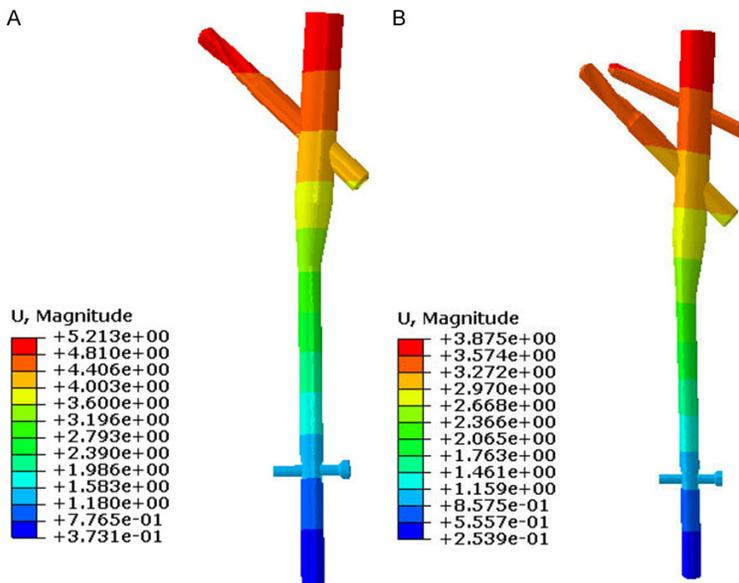
**Figure 6.** Displacement distributions on nails in two types of fixation groups. (A) PFNA fixation group, (B) improved PFNA fixation group.
