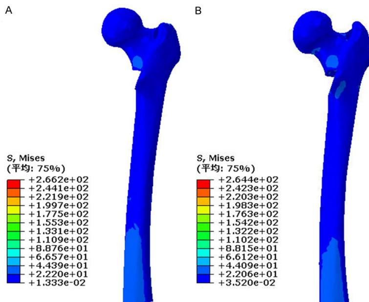
**Figure 3.** Von Mises Stress distributions on femur in two types of fixation groups. (A) PFNA fixation group, (B) improved PFNA fixation group.
