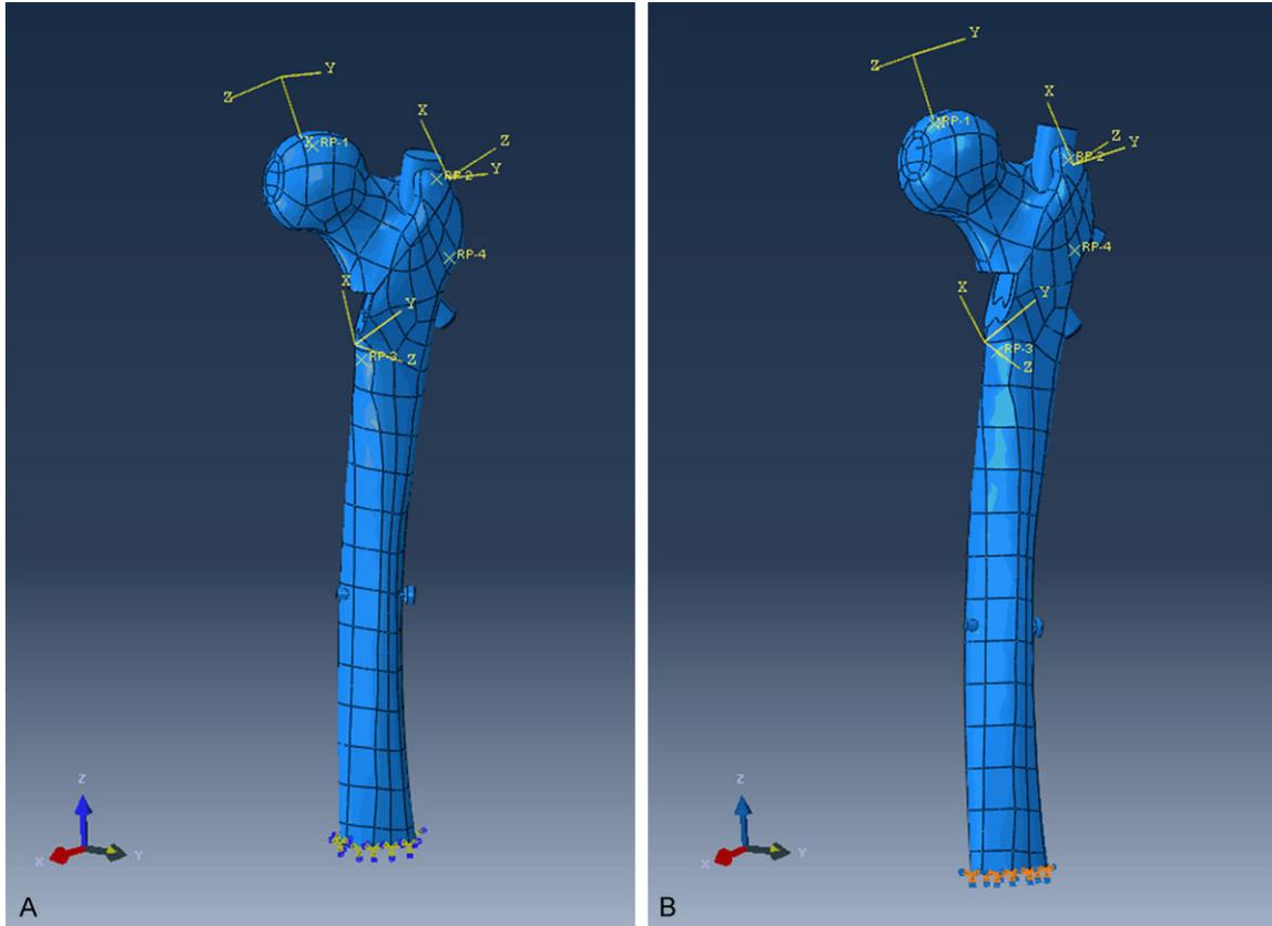
**Figure 2.** Boundary and load conditions of the two models. (A) PFNA fixation group, (B) improved PFNA fixation group.
