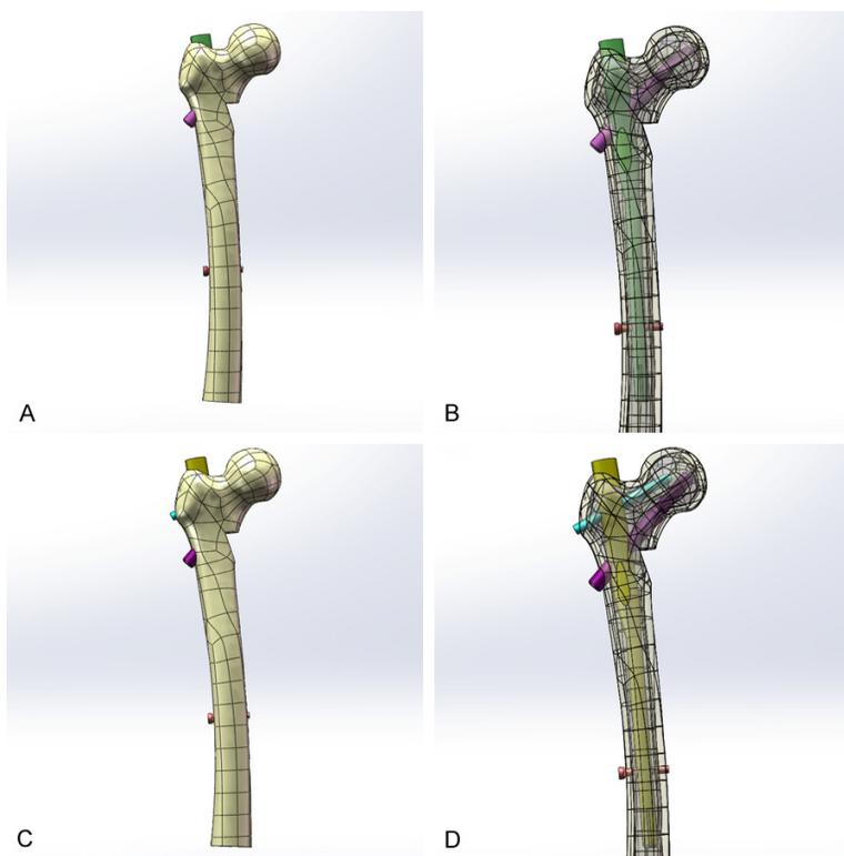
**Figure 1.** CAD models of intertrochanteric hip fracture with two types of fixation groups. (A, B) PFNA fixation group, (C, D) improved PFNA fixation group.
