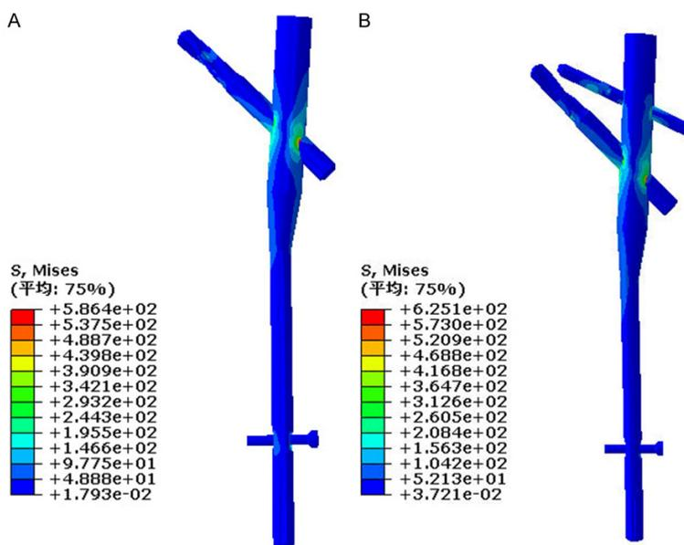
**Figure 4.** Von Mises Stress distributions on nails in two types of fixation groups. (A) PFNA fixation group, (B) improved PFNA fixation group.
