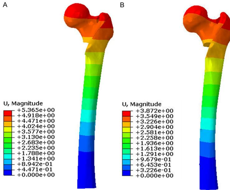
**Figure 5.** Displacement distributions on femur in two types of fixation groups. (A) PFNA fixation group, (B) improved PFNA fixation group.
