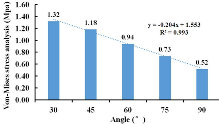
**Figure 1.** Von-Mises stress analysis at five different tilt angles. Under 200 g of horizontal force, the implant's stress decreased with the increasing of angle.
