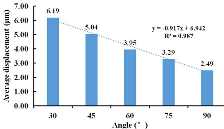
**Figure 2.** Mean displacement analysis at five different tilt angles. Under 200 g of horizontal force, the mean displacement of the implants decreased with the increasing of angle.
