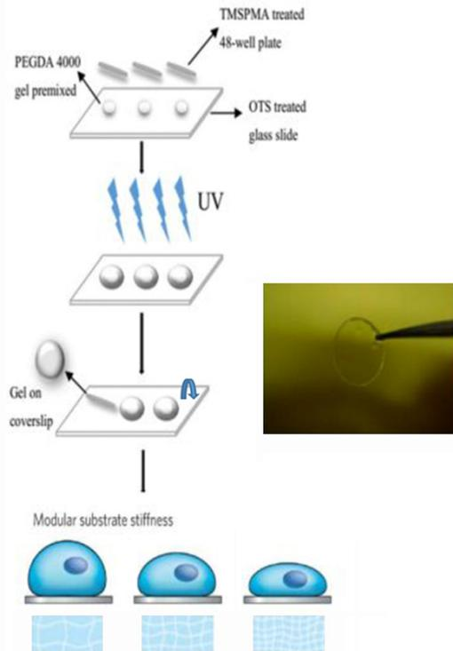
**Figure 1.** Schematic of the PEGDA hydrogel fabrication protocol. Prepolymer solutions of PEGDA (0%, 2%, 5%, 10%, respectively) were polymerized for stiffness gradient hydrogel substrates system.
