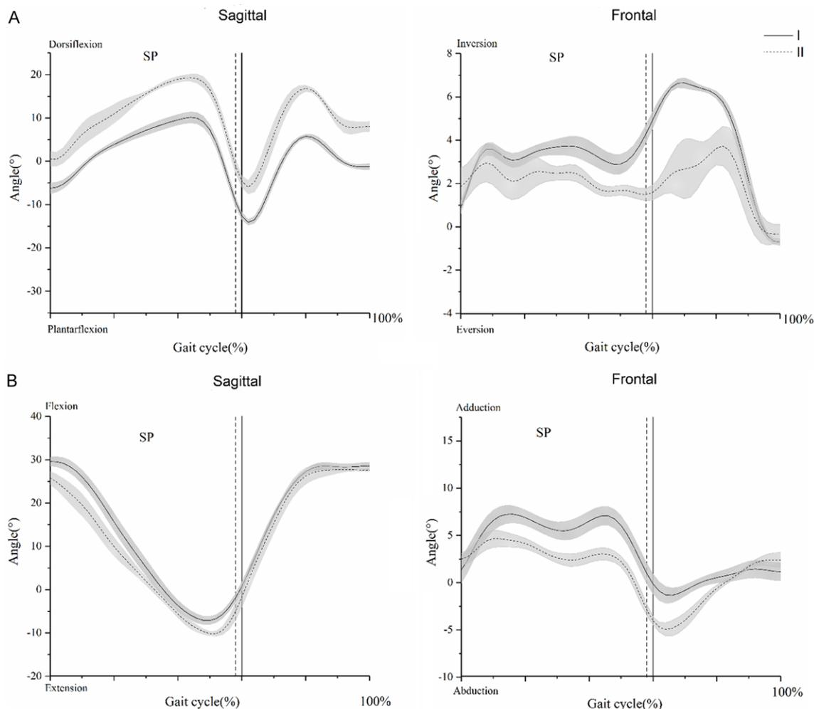
**Figure 3.** Mean angle with standard deviation curve of ankle (A) and hip (B) during a gait cycle in sagittal and frontal plane (I-solid line, II-dashed line, SP-stance phase).
