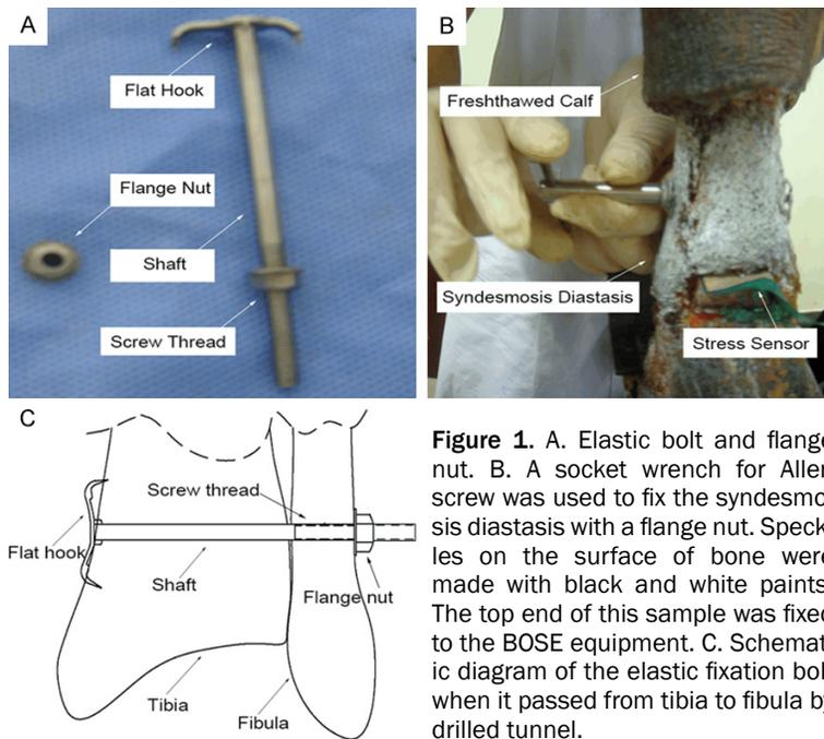
**Figure 1.** A. Elastic bolt and flange nut. B. A socket wrench for Allen screw was used to fix the syndesmosis diastasis with a flange nut. Speckles on the surface of bone were made with black and white paints. The top end of this sample was fixed to the BOSE equipment. C. Schematic diagram of the elastic fixation bolt when it passed from tibia to fibula by drilled tunnel.
