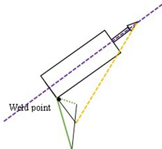
**Figure 9.** Diagram of the calculation of the vertical arm. Yellow line: cortical bone. Purple line: axis of the screwdriver. Green line: vertical arm of the locating rod.
