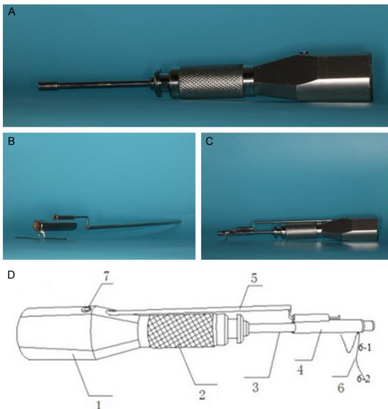
**Figure 5.** Diagram of the traditional screwdriver and modified screwdriver. A. Traditional screwdriver. B. Auxiliary positioning attachment. C. Modified screwdriver tip. D. The assembly of the modified screwdriver. (1 Hand shank, 2 Roll booster, 3 Fixed link, 4 Drive pipe, 5 Connecting rod, 6 Locating rod, 6-1 Vertical arm, 6-2 Horizontal arm, 7 Screw).
