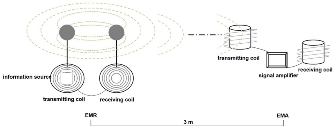
**Figure 1.** Experimental device schematic diagram. The device was composed of an EMR and EMA apparatus. The transmitting coil of EMA was 3 m away from the receiving coil of EMR.
