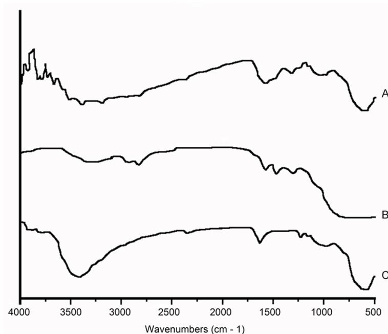
**Figure 2.** Infrared spectrograms for  $\text{Fe}_3\text{O}_4$ , polyethyleneimine (PEI) and PEI-coated  $\text{Fe}_3\text{O}_4$  nanoparticles. A. PEI-coated  $\text{Fe}_3\text{O}_4$  nanoparticles. B. PEI. C.  $\text{Fe}_3\text{O}_4$  particles.
