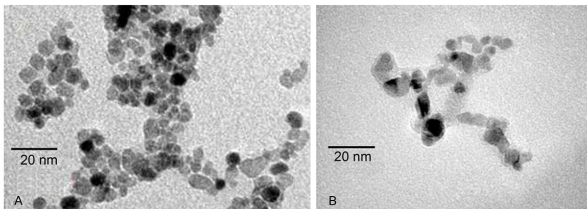
**Figure 1.** Transmission electron micrograph. A.  $\text{Fe}_3\text{O}_4$  nanoparticles. B. Polyethyleneimine (PEI)-coated  $\text{Fe}_3\text{O}_4$  nanoparticles.
