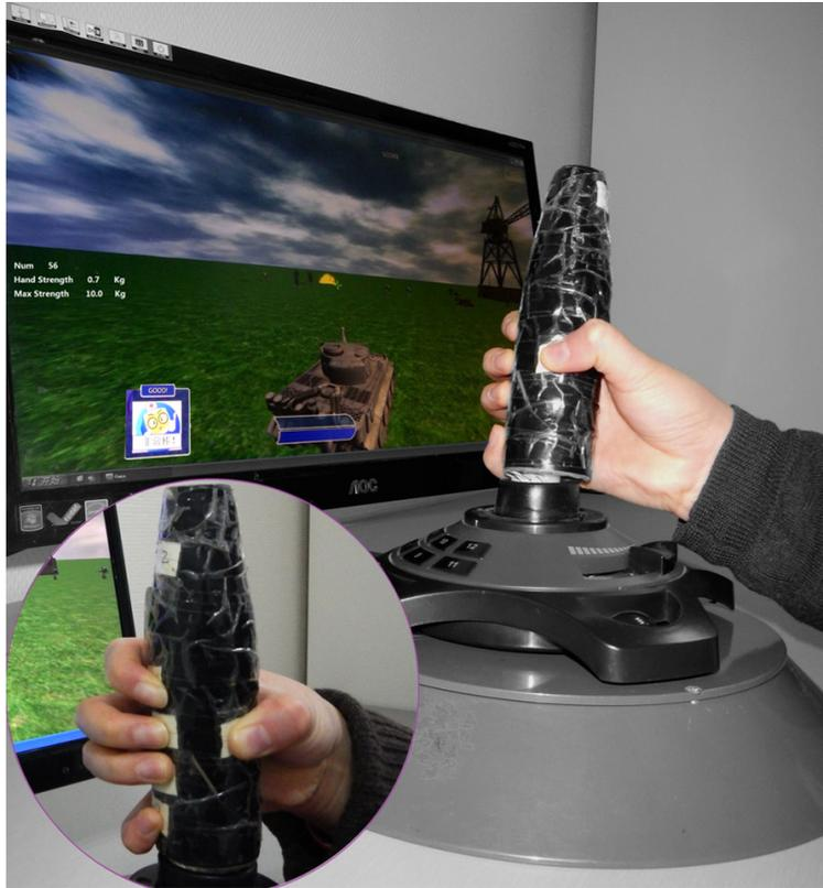
**Figure 1.** A subject is using the computer-assisted wrist/hand training apparatus. The photograph at bottom left shows the locations of force sensing resistors (FSRs).
